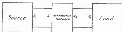
FIG. 2 Relation of attenuation network to the source and the load. Usually the network is so designed that Z_s = Z_1 and Z_L = Z_2 .
